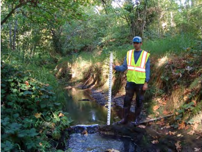
Hard clay forming pools within channel bed in Saum Creek Reach #2 (photo location shown below with camera icon)
