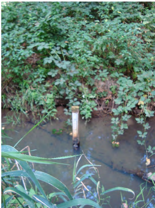
Site location: 100' upstream of SW Tualatin-Sherwood Road Photo number: H2-2 Description: Staff gauge in channel
