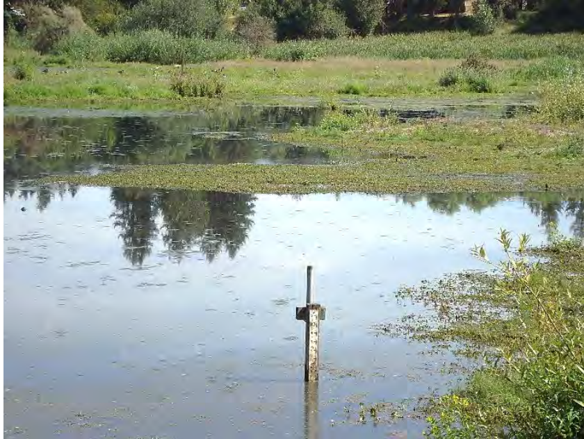
Site location: Nyberg Wetlands, downstream side of beaver dam Photo number: N2-3 Description: Staff gauge in ponded area
