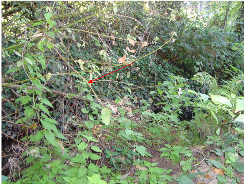
Site location: 500' upstream of SW Tualatin-Sherwood Road Photo number: H2-5 Description: Debris on branches above channel (~4') indicating high water mark (red arrow)
