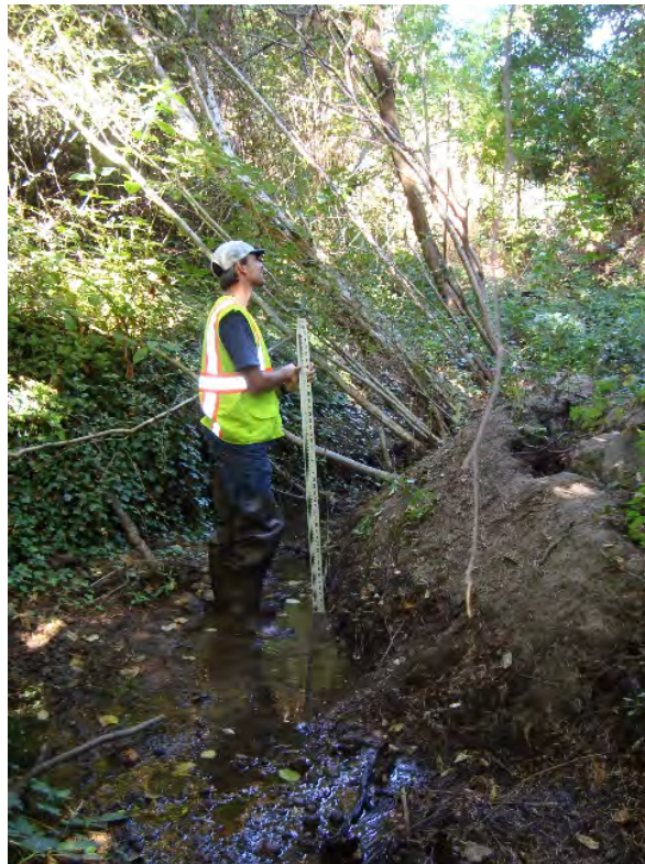
Site location: 600' upstream of confluence with S. tributary Photo number: H3-26 Description: Left bank slumping
