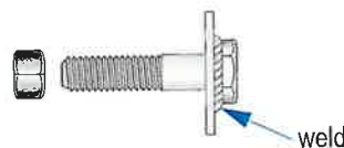
Mounting Pin Welded Assembly, Qty (12) Weld bolt to washer as shown Weld nut to wall frame GG&V #6000080: 5/8-11nc x 3" Bolt SS GG&V #6000071: Flat Washer SS 3/4" id x 2"od x 1/8" GGV #600070: 5/8" Grade 8 Nut NO SCALE
