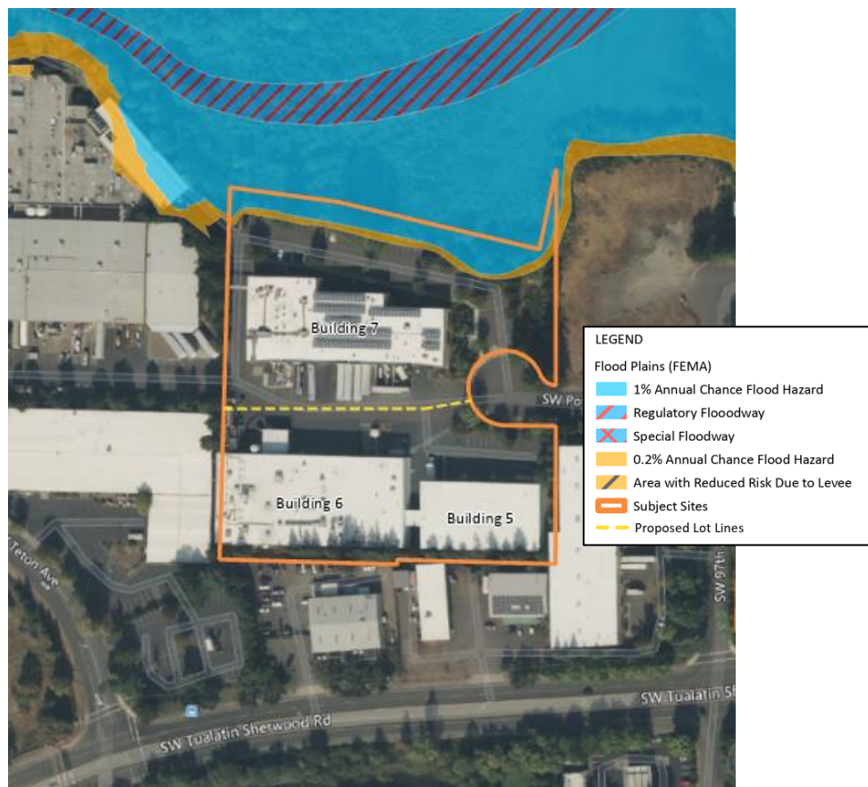
Figure III-1. Site and FEMA Flood Hazard Areas
